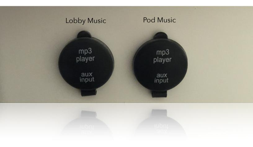
A) Pod Music Audio Port: You will need to run a 3.5mm male-to-male shielded headphone cable from the back of the pod, to the bench area or custom docking station in the room. One end will plug into their device and the other end will plug into the back of the pod.
